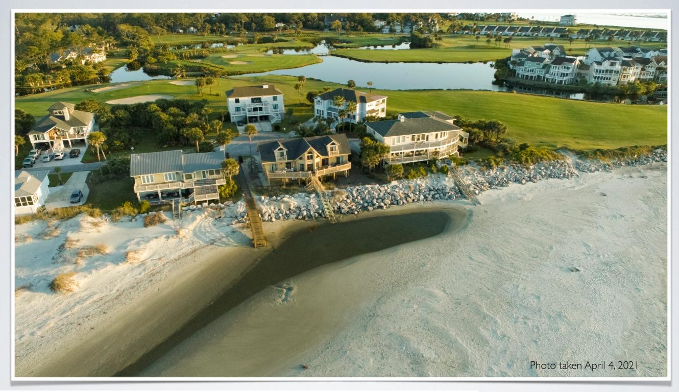
Access #1b - This photo, taken at low tide shows the beach access stairs end at the muddy sediment near the edge of the tide pool. As the pool drains, this pluff mud remains at the base of the stairs leaving a very slick surface with which to step down onto the beach. The beach sand in front of the tidal pool has filled back in and is at a much higher profile than the area around the tidal pool leaving the only drainage direction back towards where the water originally flows in.
