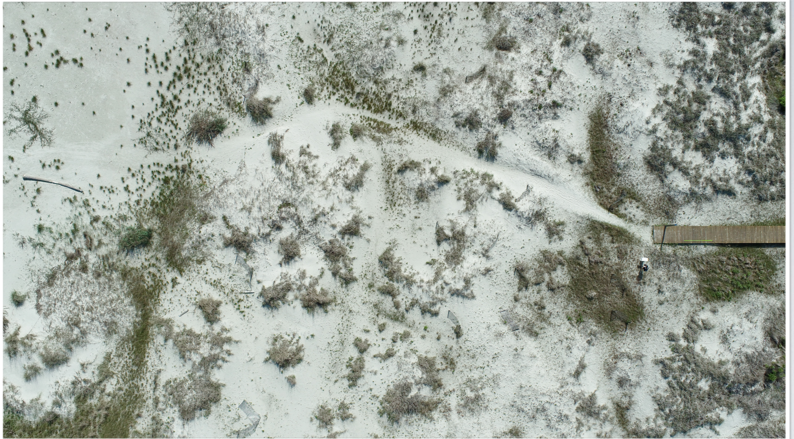
Access #6 - Beach access #6 ends a considerable distance short of the beach. As a result, the meandering foot path carves its way through two smaller dune lines and vegetation.
