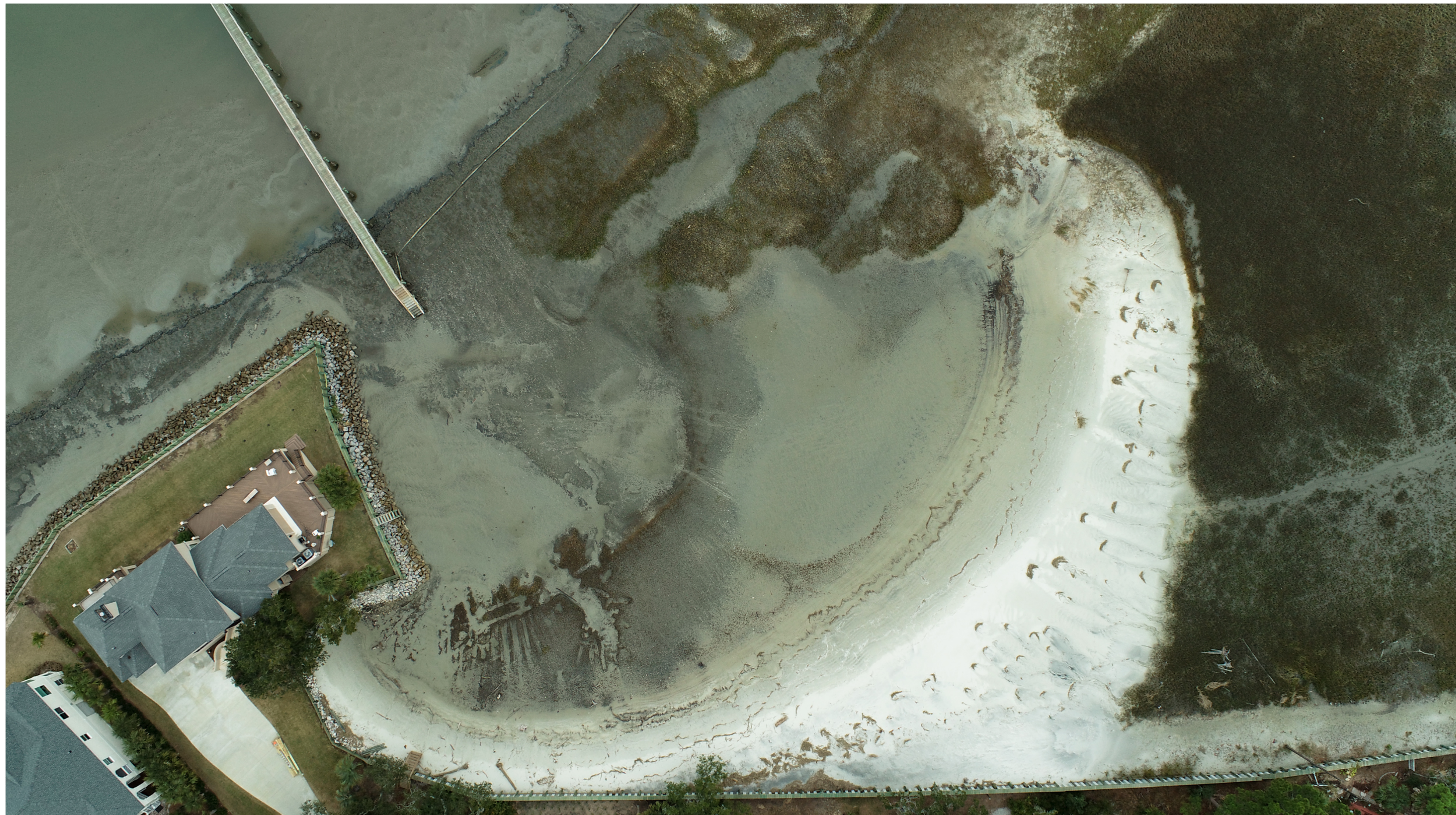
This aerial photo, taken at low tide taken on January 21, 2022 , shows the eroded area is expanding rapidly and is now easily, two to three times the size of the entire property footprint of the Mollura residence.
