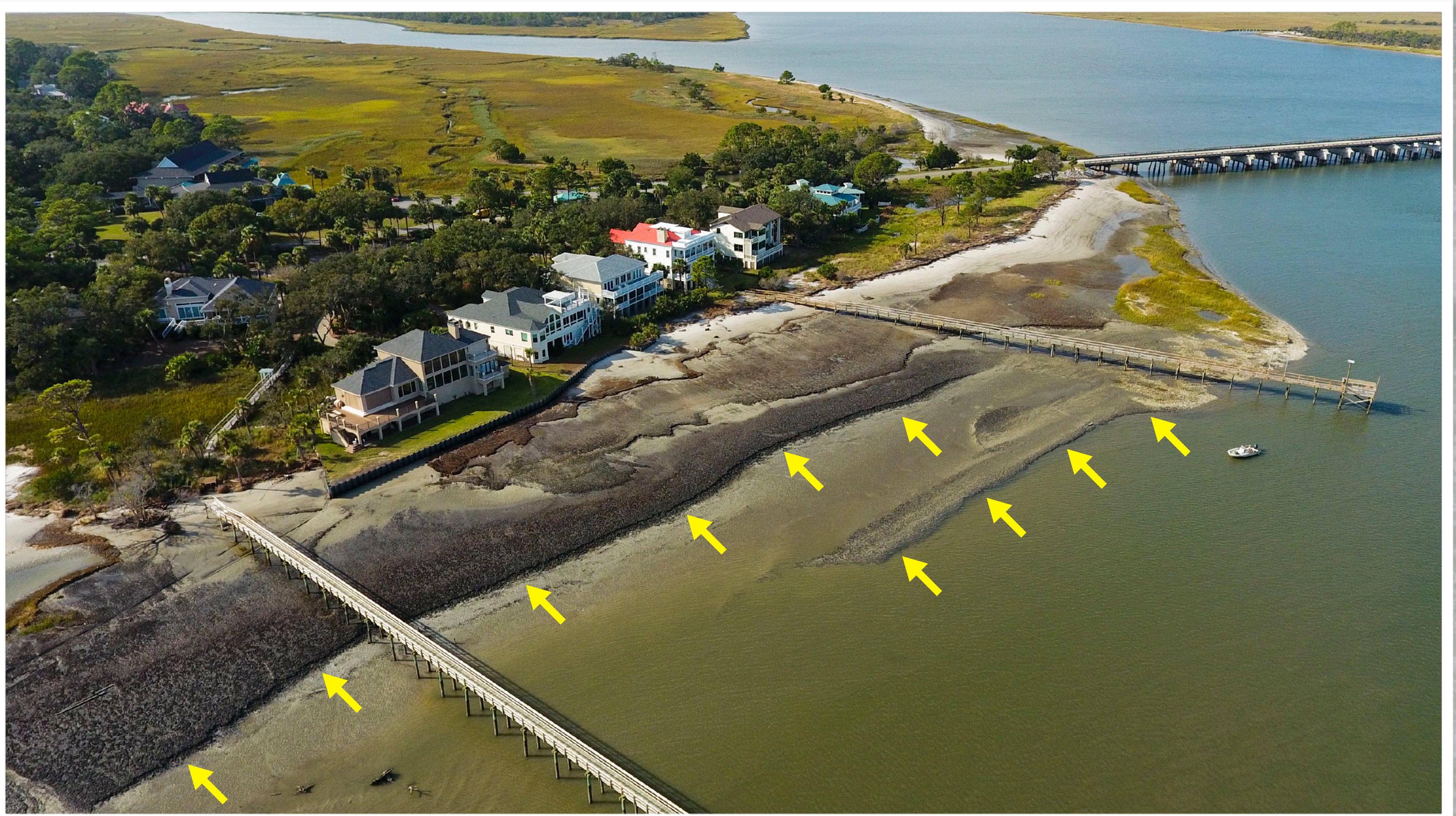
In this view, taken at low tide on November 6, 2018 , the line of soil minus the vegetation is visible. Much of the vegetation had already been eroded away leaving only the soil footprint remaining. Left unprotected, the soil is quickly eroded by both wave action and the tidal flow that occurs in the inlet.
