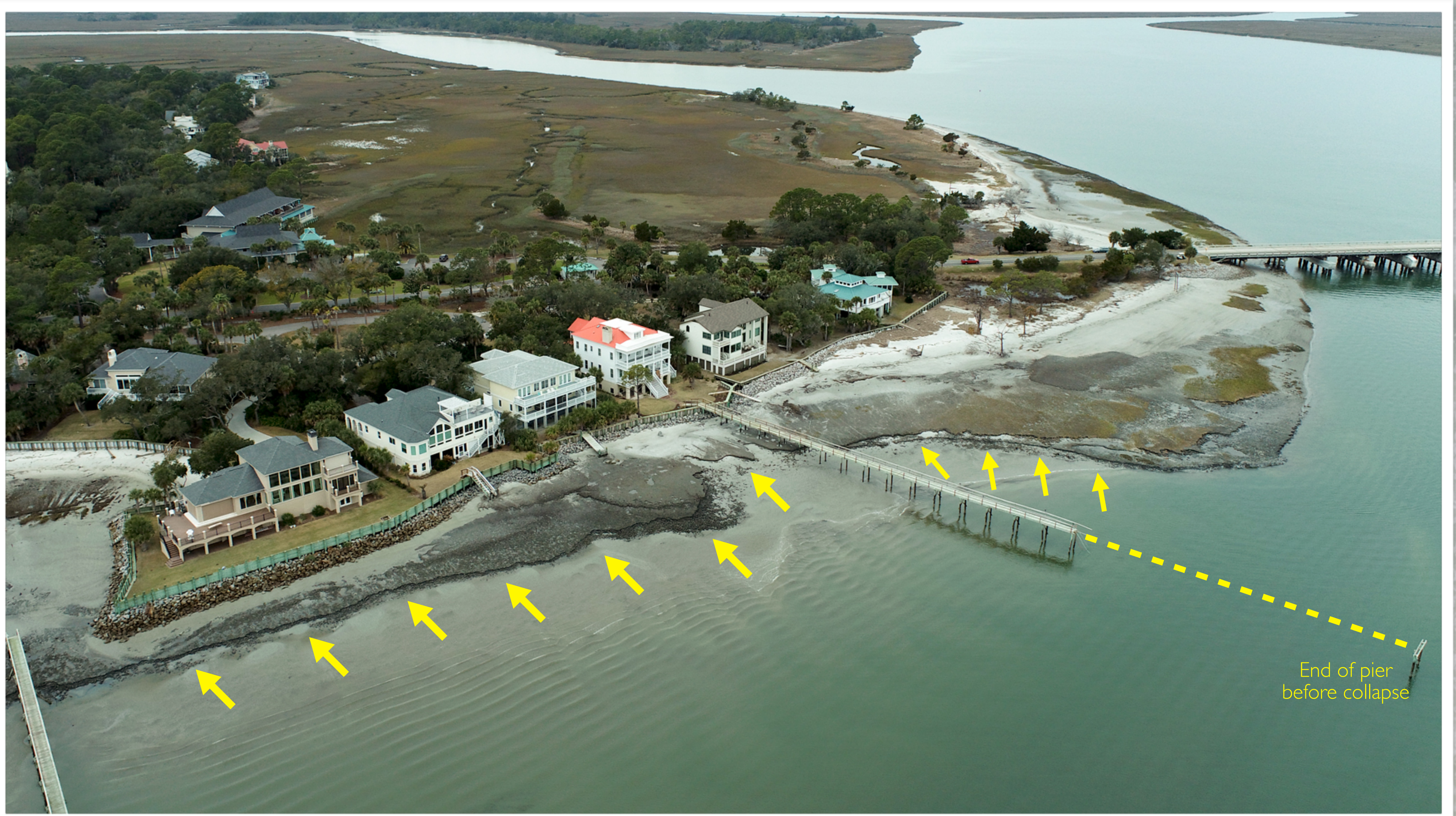
This photo taken three years later, on January 23, 2022 , shows the extent of the erosion of the unprotected soil starting at Wardle's pier and moving past the River Club pier towards the front of the salt marsh. This area gets hit by both wave action and tidal currents.
