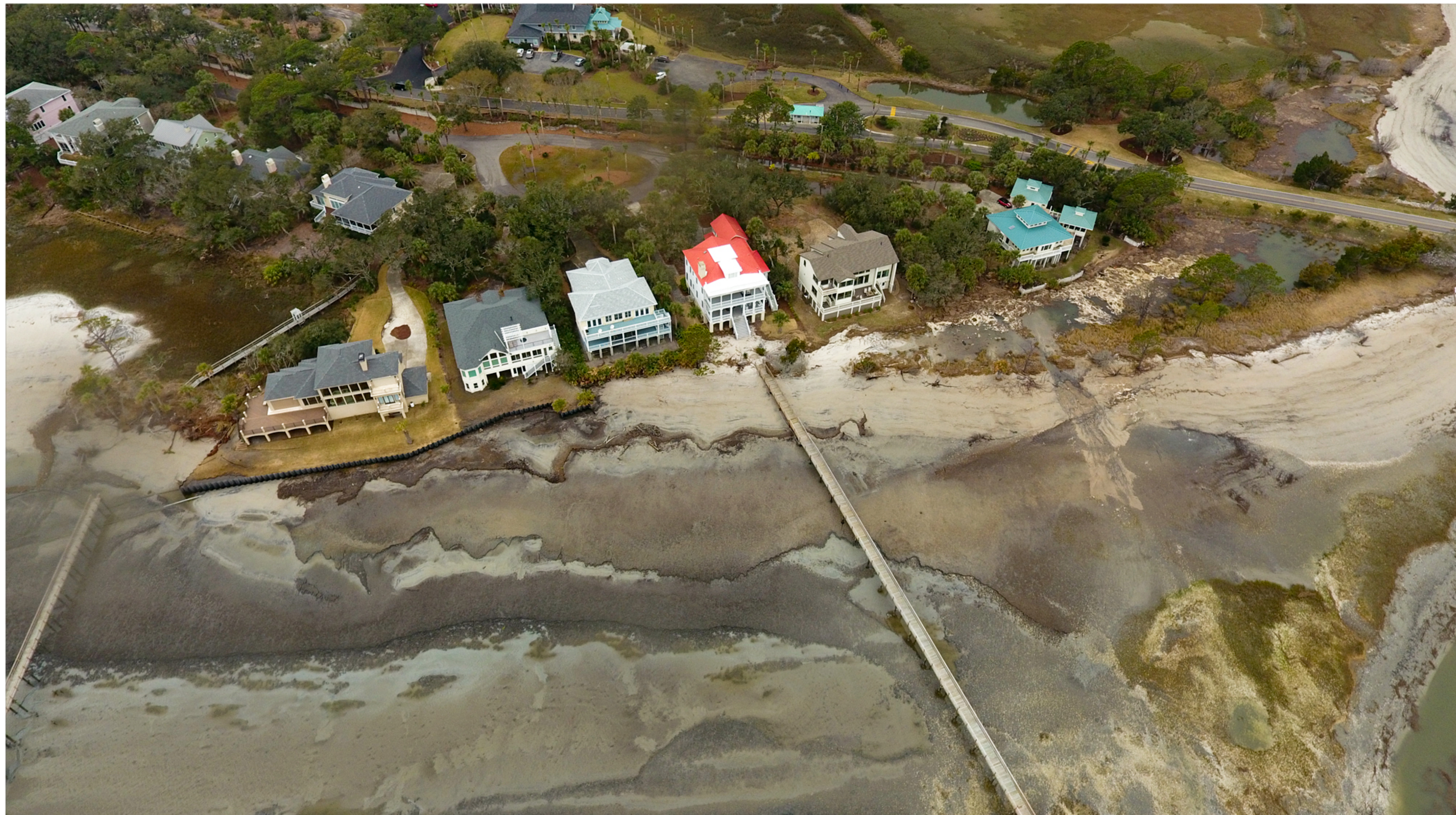
This photo, taken at an extreme low tide (during a king tide cycle) on February 20, 2019 , shows several layers of underlying soil. The sea-facing hard edge of the layers indicates fresh erosion with each flood cycle, which can be seen in the next slide.
