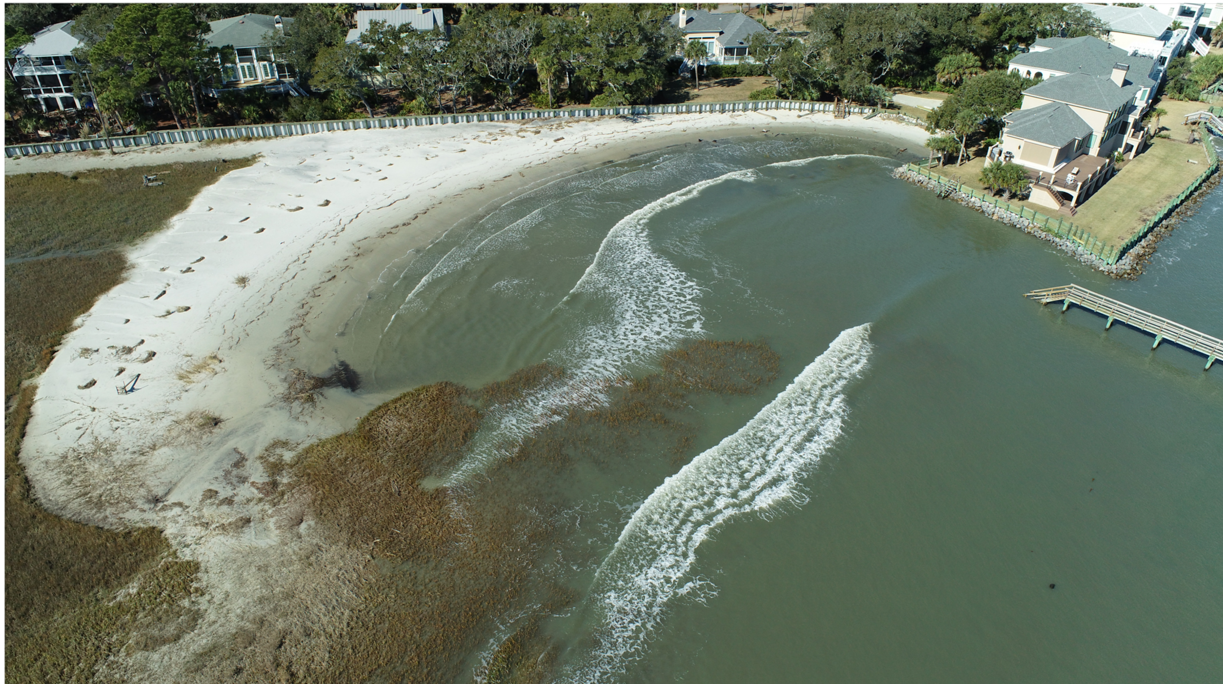
A good illustration of how spartina grass in the salt marsh helps control wave action. In the large opening, waves reach the sandy area at or near full strength, but the wave energy flowing through the grass is dispersed quickly and has almost no force left shortly through the grass.
