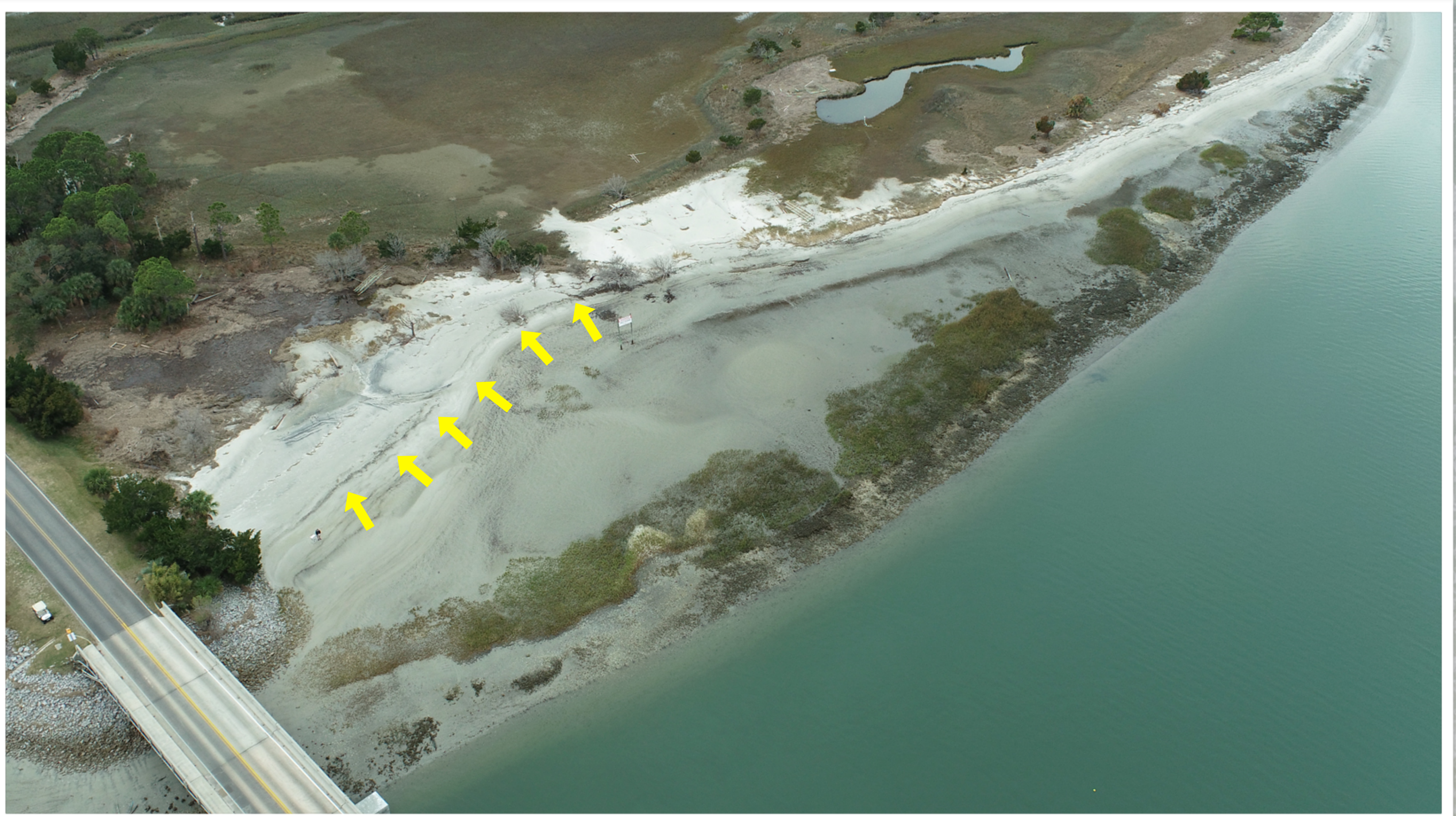
This photo, taken at low tide taken on January 20, 2022 , shows the breached area has joined the existing eroded area next to it, creating a larger sand-only footprint that continues to expand along the bridge approach and throughout the whole area.
