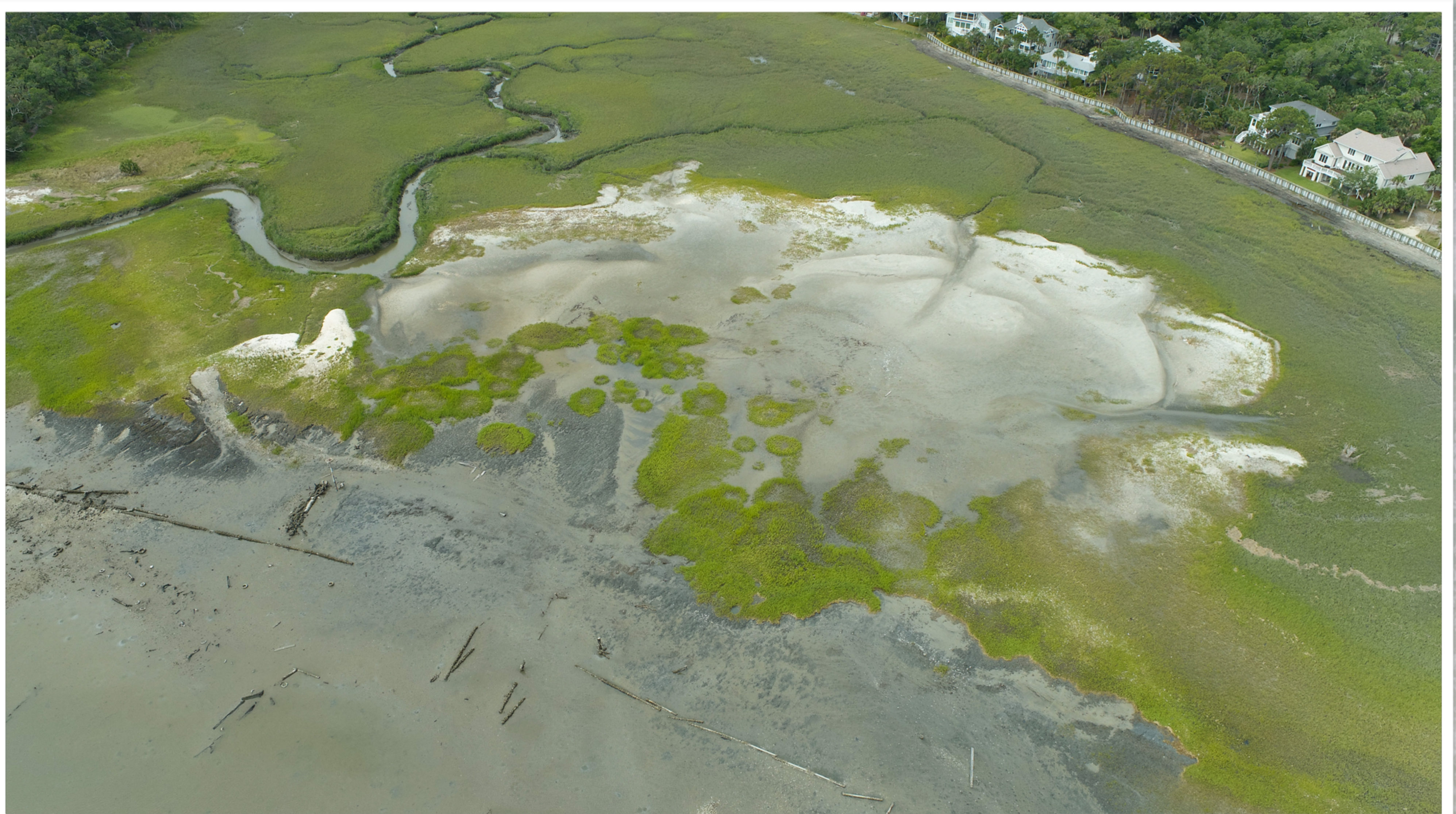
Salt marsh behind River Club - Vegetation has started to grow on the exposed clumps of mud showing the marsh still has a chance to repair itself. At the same time a note of reality, the old utility pipes now exposed were once buried several feet underground which shows how much material has been pushed back into the marsh by the wave action.
