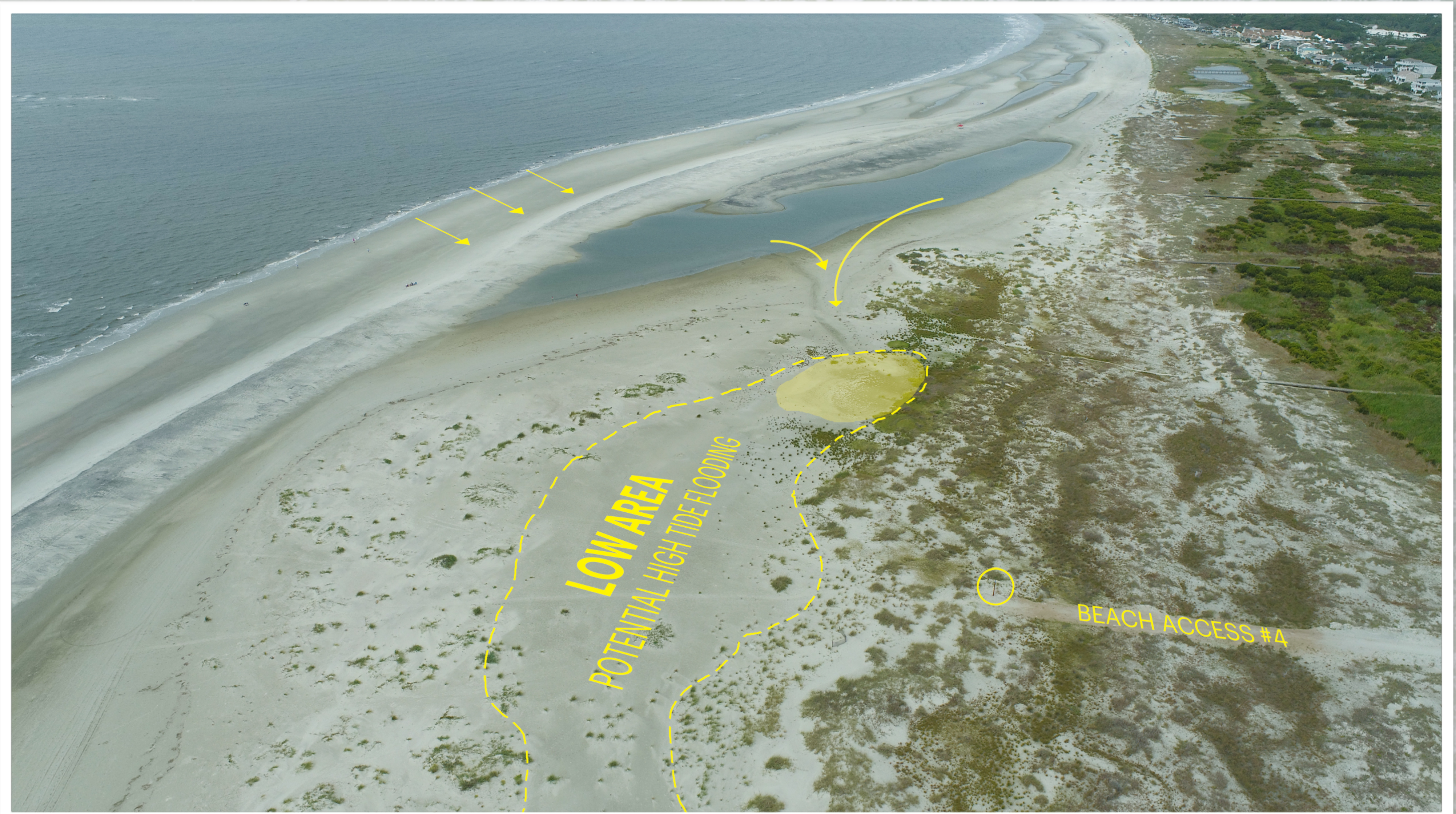
King tide activity - The May 24th king tide pushed sand ashore squeezing the tide pool which caused the water to spill into the low lying area at the end of access #4. The shaded yellow is as large as the overflow water got, but the whole dotted line area is currently susceptible to tidal flooding.
