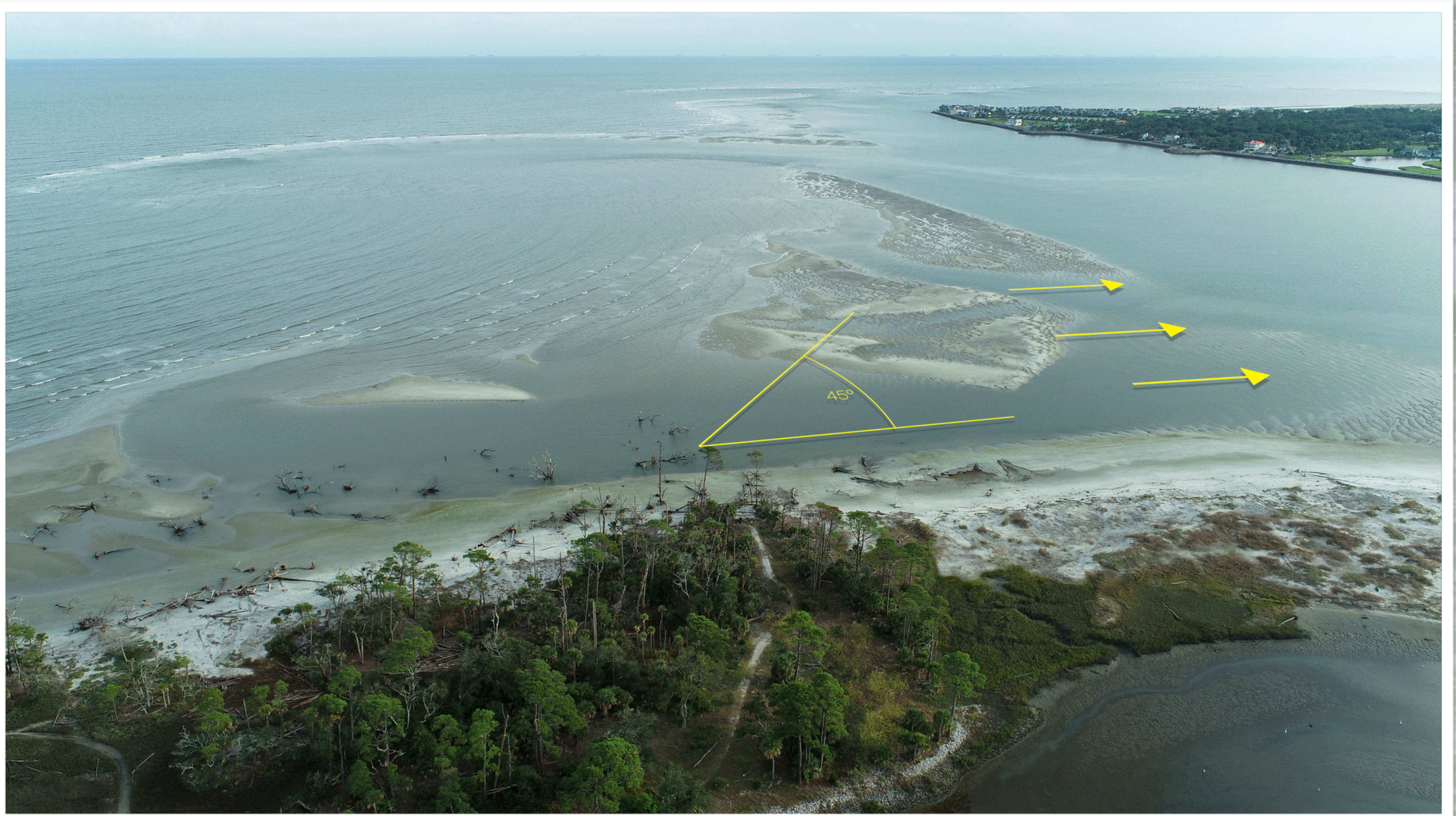
The Littoral Current - When waves strike the land mass at an angle, as seen here, it creates a flow called a littoral current that runs parallel to the shoreline. This is a natural distribution of sediment along a beach. Here, the sand is being pushed into the inlet and the current carries it out around the front of Fripp Island.
