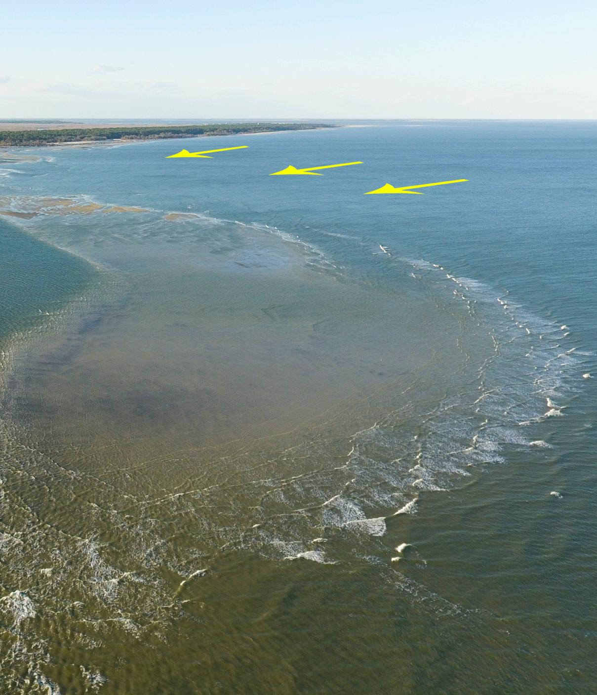
As the sand pushes against the immoveable rock revetment, it squeezes the channel opening which increases the velocity and, in turn, the depth of the inlet. Any sand or sediment that gets pushed into the current is immediately flushed out of the inlet due to the increased flow rate.
