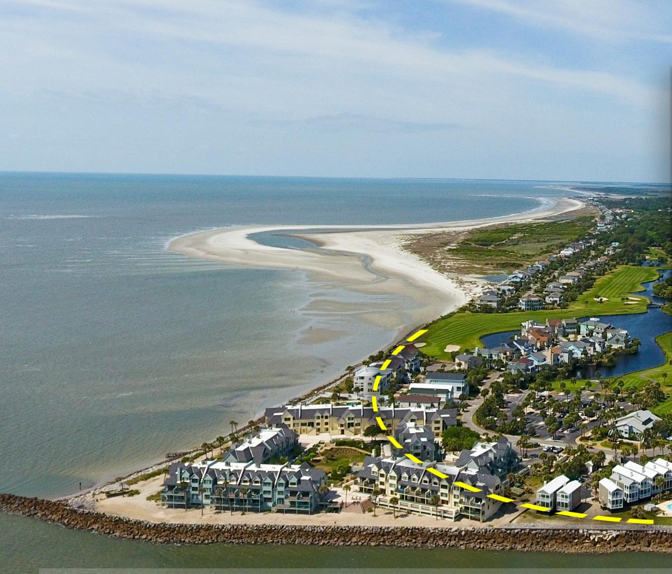
The northern tip of Fripp Island is protected by a rock revetment so the rounding doesn't occur. If the same sawing motion were to occur to an unprotected side of Fripp Island, the damage would be catastrophic to a large number of homes.
