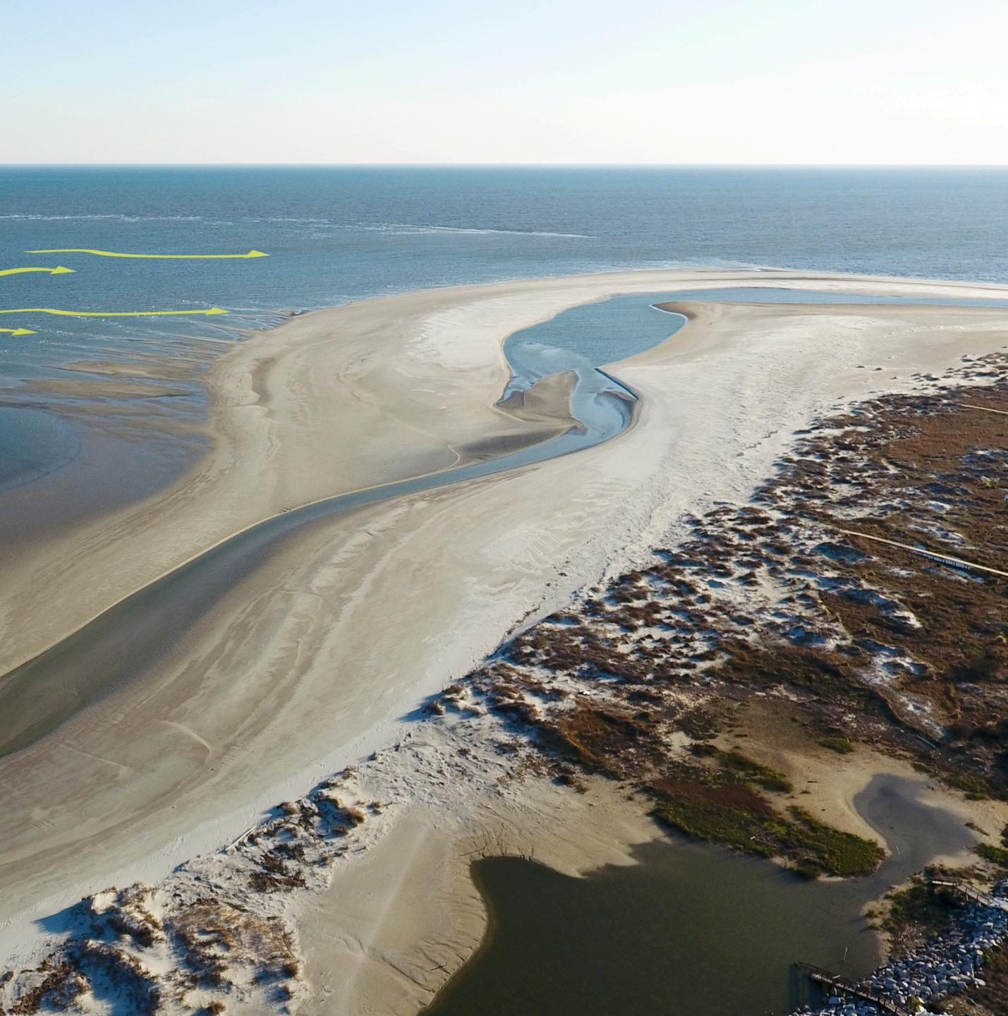
This outer ring marks the spot where the current, flowing out from the inlet meets up with the waves that push towards the beach. The weakening current runs out of energy and is not strong enough to block the sand so it forms a natural arc of sand as the beach-wards moving current eventually overpowers the southflowing current and the sand is pushed towards the beach.
