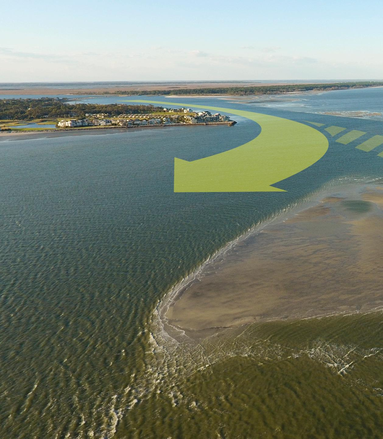
The south moving sand can't compress the channel any narrower due to increased velocity. Once it clears the revetment it continues its southward push forming an elbow out in front of the island and fills in the once straight-flowing channel. This changes the direction of the outward flowing inlet
