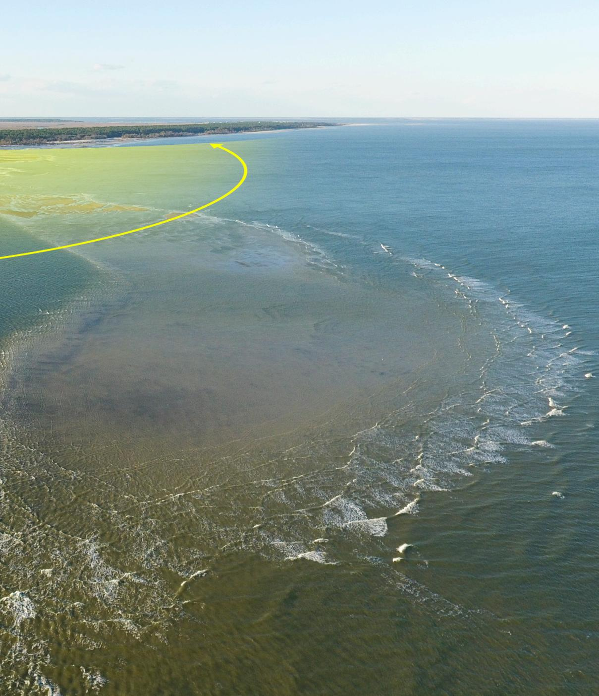
Another source of sand is the naturally occurring littoral drift that moves south across the face of Hunting island. All the sand builds up parallel to the rock revetment forming a shoal in the middle of the inlet.
